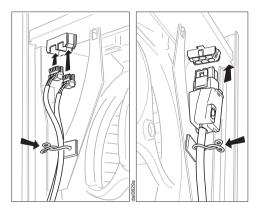
Plug the connectors on the canopy into the corresponding receptacles left and right of the motor assembly.
